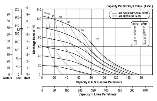
NOTE: Performance based on the following: PTFE fitted pump, flooded suction, water at ambient conditions. The use of other materials and varying hydraulic conditions may result in deviations in excess of 5%.
